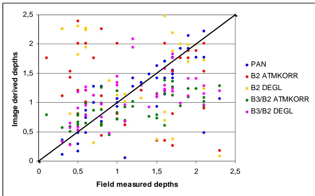
Figure 9. Image derived depths compared to field measured depths.
