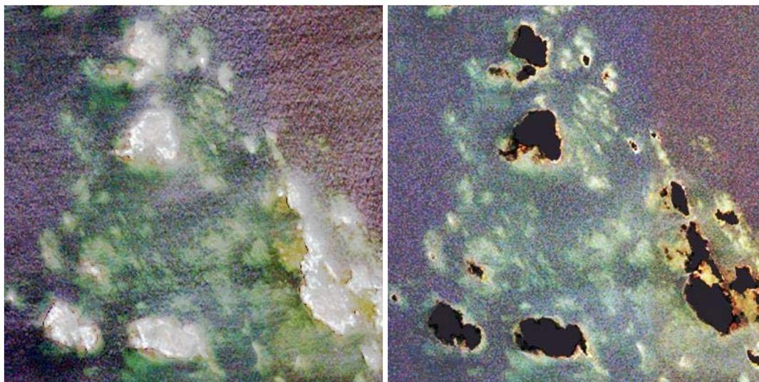
*Figure 3a and b. Islands and subsurface areas before (3a) and after (3b) the sea surface correction algorithm has been applied.*
