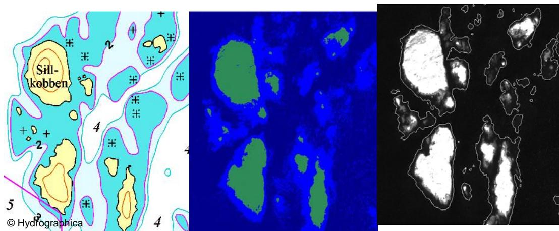
Figure 13a-c. The figure shows a part of the nautical chart from Hydrographica, the corresponding QB-PAN area and a possible 2-meter vector product.
