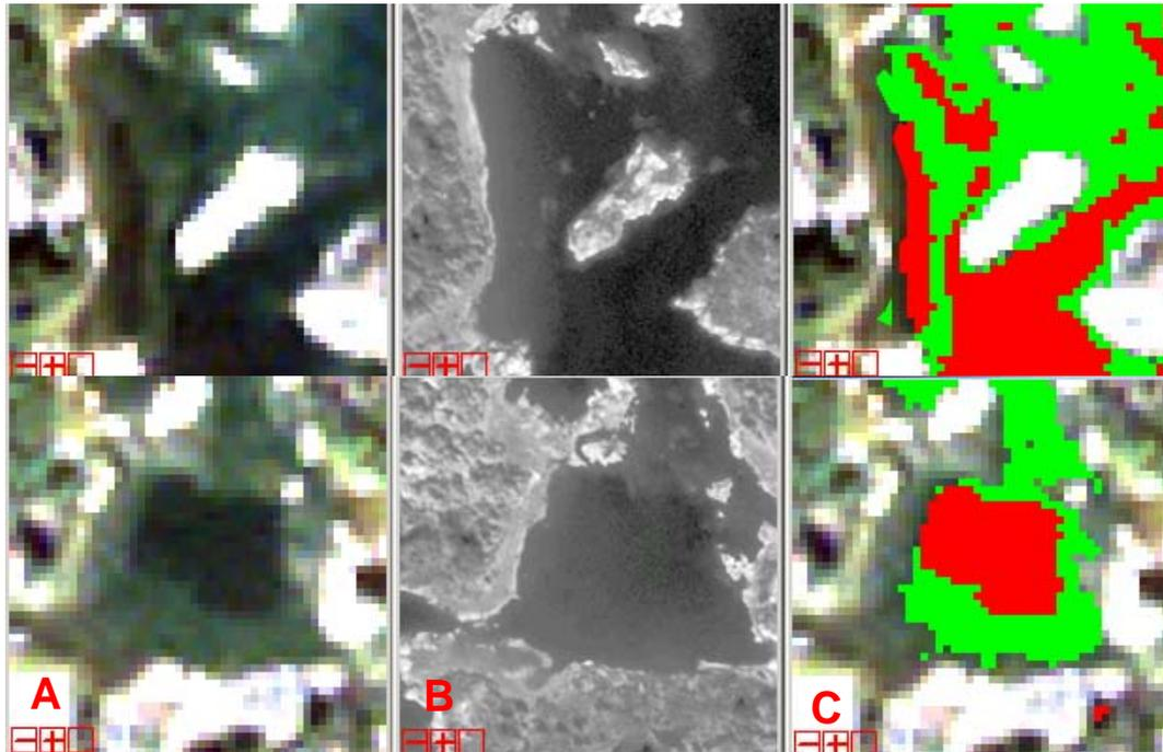
Figure 21a-c. (a) The multispectral image from August, (b) the panchromatic image from May and (c) vegetation covered areas in red, identified in August.
