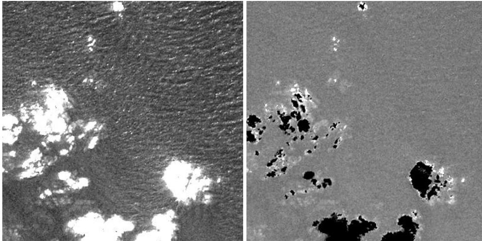
Figure 4a and b. Söder-Gåsgrund, east of Gräsö, before and after the sea surface correction algorithm has been applied.
